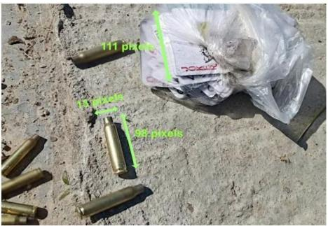
Figure 21: Pixel-ratio analysis indicates a rough specification of the cartridge. The calculation was based on standard playing card dimensions, where 111 pixels = 64mm; 1 pixel = 0.5766mm; therefore Cartridge length = 56.5mm and Cartridge shell width = 7.5mm. Minimum error is +/-0.5766mm though due to perspective, will be greater.
